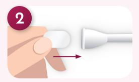
Put one insert in the space provided at the end of the applicator. The insert should fit snugly and not fall out.
